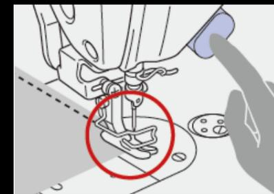
Easier reverse sewing operation with the handy switch than before, it was done with the reverse lever. The switches are located within operator's grasp, operator can be done the operation without slowing down the operatability.
