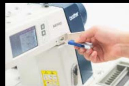
The USB port is equipped so sewing patterns and environmental settings can be copied easily to other sewing machines. Also, you can upgrade the software with USB memory.
